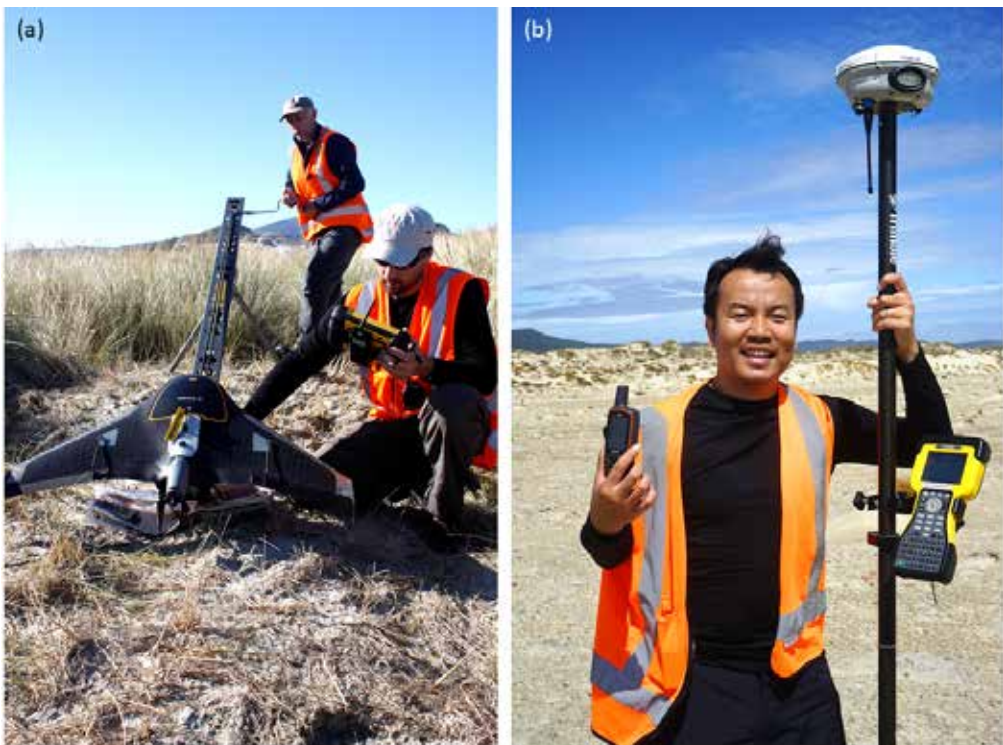
Figure 45: RPAS (or UAV (drone)) technologies are now used to derive orthophotographs and digital elevation models. The first RPAS survey was completed by the staff of the School of Surveying in April 2015 (a) - here launching the Trimble UX5 RPAS from the Mason Bay foredune. Subsequent aerial surveys have used a Phantom 4-Pro UAV quadcopter. PhD candidate Nguyen Minh Duc (b) is using a hand-held Garmin 62S GPS and an RTK-GPS to establish ground control points prior to a UAV survey (November 2018).
